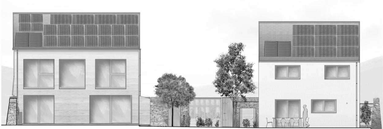
**Figure 4: (left) Larch House 55% south glazing and (right) Lime House 20% south glazing; as built using extreme 10 year worst case Ebbw Vale weather data**
