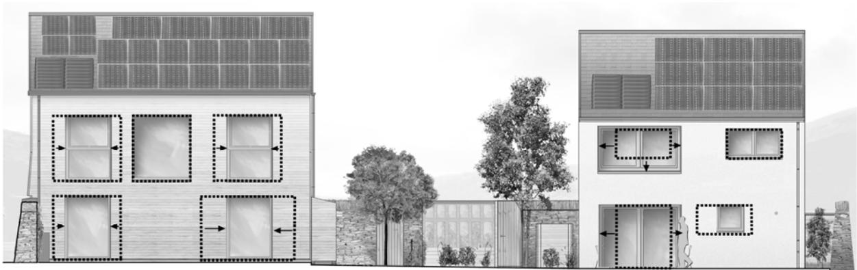
**Figure 5: (left) Larch House 33% south glazing and (right) Lime House 33% south glazing; redesigned using only Manchester mean weather data which also allows a cheaper fabric specification**
