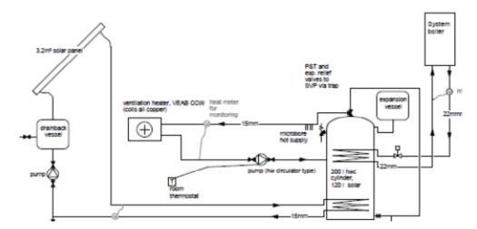
Here the coil temperatures proved more critical, as we require 100% air heating from water at standard dhw storage temperatures of around 55°C. The larger capacity heater battery was fitted and this provides air at 49°C for water flow and return temperatures at the heater of 53°C/46°C and cylinder set point of 55°C.
