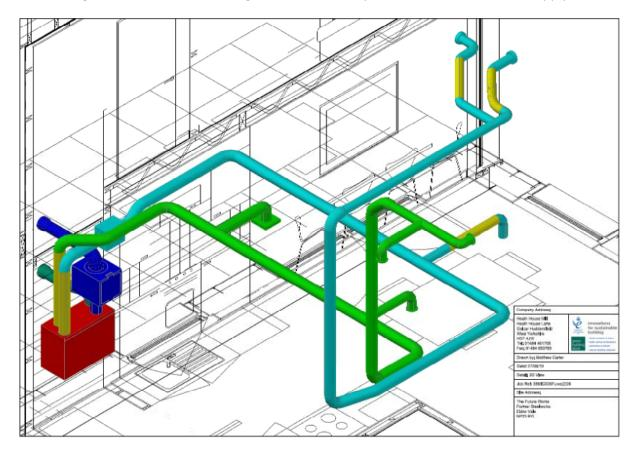
Ducts have to run in the first floor to get around the staircase before rising in the airing cupboard to serve bedrooms and bathroom via a lowered ceiling void as in Larch house.
