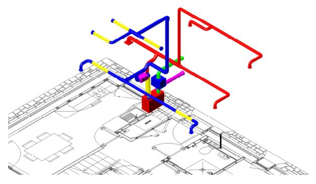
Ducts run in a limited zone between joists to kitchen dining shower room and living areas and rise in the airing cupboard to run in lowered bathroom and landing ceilings. Bedroom supply terminals are wall mounted and the ceiling is higher in bedrooms.
