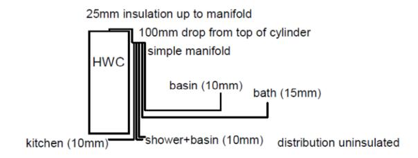
The same distribution type is used in both houses. Cold water distribution is normal, using 15mm pipework.
