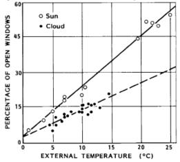
In each of the spaces which have windows, one typical window is chosen. Actually only the kitchen has the windows, whereas all other spaces have sliding/tilting doors. Thus, aforementioned function related to the external temperature is applied to the kitchen window, due to its reasonable size. For control of window opening by external temperature in TAS zdcem function is used.
