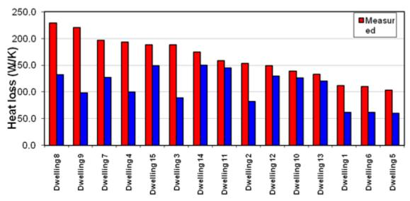
Figure 5- Measured and predicted whole house heat loss in 16 new low energy dwelling (Wingfield, et al., 2009, cited in GHA, in press, p. 25)
