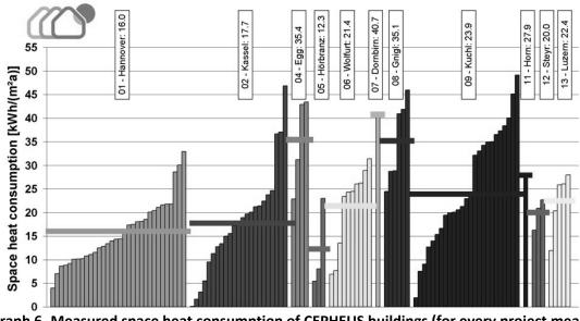
Graph 6- Measured space heat consumption of CEPHEUS buildings (for every project mean is displayed as a horizontal bar) (Schnieders, 2003, p. 345)
