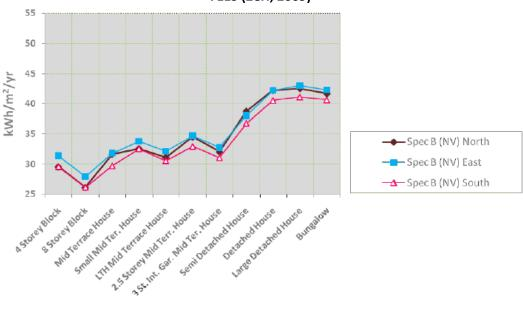
Considering that site constrains can be restricting in terms of use of optimal orientation, the model of the house is rotated in order to estimate maximal variations in heating demand. Variations in cooling load are not within the scope of this study but they are expected to be minimal compared to heating due to use of shading.
