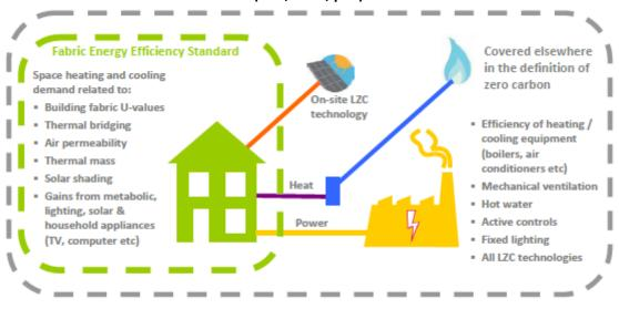
Figure 2- Task group definition of the scope of the Fabric Energy Efficiency Standard (ZCH, 2009, p. 8)
