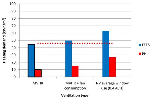
Graph 11- Comparison of MVHR ventilation with natural ventilation with the same effective ventilation rate of 0.4ACH
