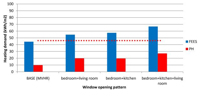
Such results indicate that even in case of the most modest window use, the FEES heating load limit would be exceeded and more energy would be consumed than in case of MVHR. Furthermore, it is becomes clear that use of obligatory use of MVHR within the Passivahaus standard significantly contributes to such low levels of heating demand which can hardly be achieved with natural ventilation.
