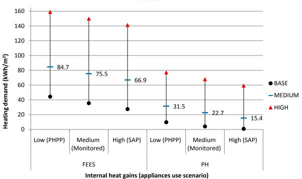
Graph 30- Effect of internal heat gains on heating demand of FEES and "PH house" with natural ventilation
