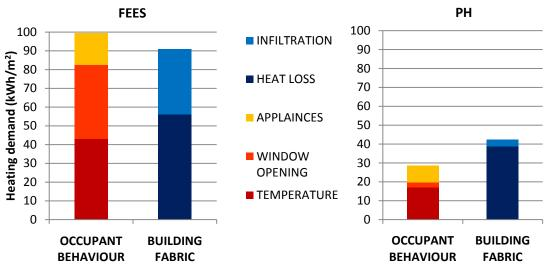
Graph 22- Comparison of estimated maximal realistic variations in heating demand due to occupant behaviour and deterioration of building fabric for FEES and PH house
