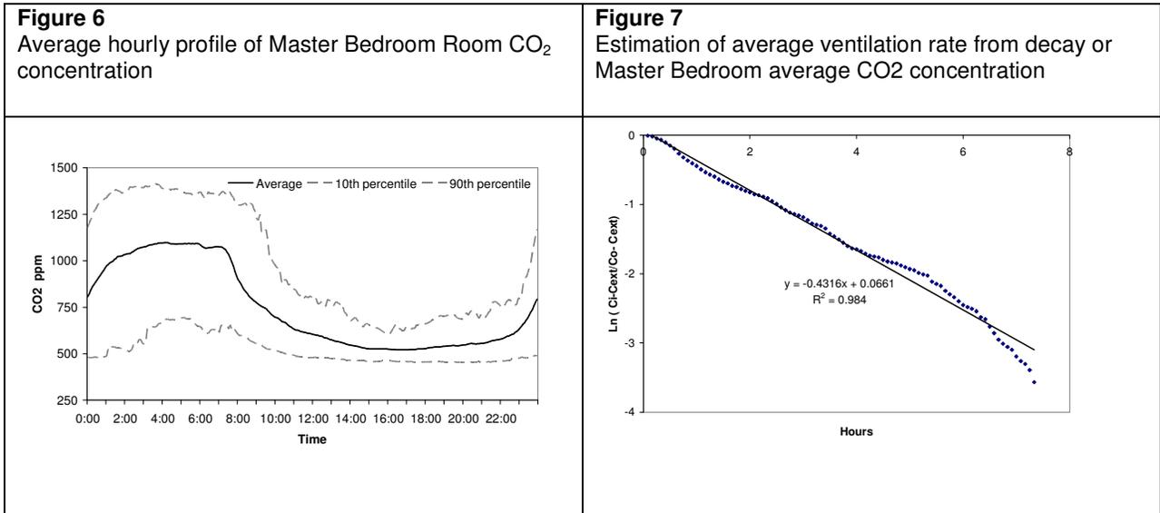
The ventilation rate measured by the CO<sub>2</sub> decay and the flow rates measured at the MVHR unit are in close agreement. The measured average ventilation rate of 32 l/s and the measured average power consumption of 36 W, results in a measured specific fan power of 1.1W/l/s or electric power consumption, P<sub>el</sub> of 0.31 Wh/m<sup>3</sup> for the MVHR system.
