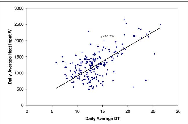
The measured average total heat loss of the building based on 182 winter days is 90.6 W/K  $\pm$  2.2 W/K (standard error in mean of Daily Input/Daily DT). With a heated floor area of 101m<sup>2</sup>, the heat loss coefficient of the dwelling is measured at 0.90W/K/m<sup>2</sup>.
